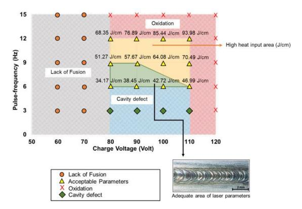
Figure 17. Adequate laser parameters.
