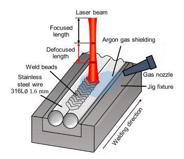
Figure 4. The schematic experimental setup.
