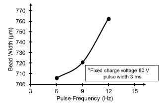
Figure 10. Effect of pulse frequency on weld bead width.
