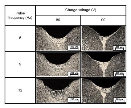
Figure 11. Cross-sectional macro structure.
