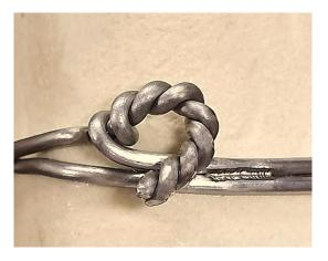
Figure 5. Cerclage wire joints with laser welded.
