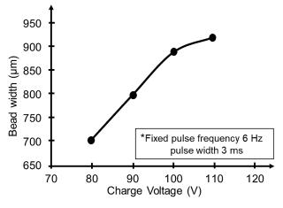
Figure 9. Effect of charge voltage on weld bead width.
