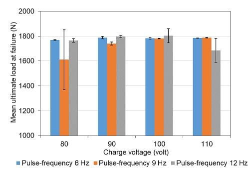
Figure 16. Effect of laser parameters on ultimate load at failure ±SD (length of welding 15 mm).
