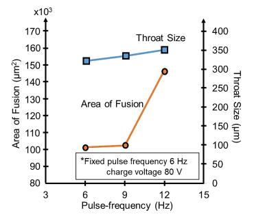
Figure 13. Effect of pulse frequency on area of fusion and throat size.
