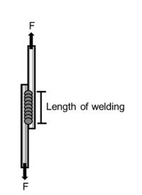
Figure 7. Schematic view of the relationship between shear loading and weld joint.
