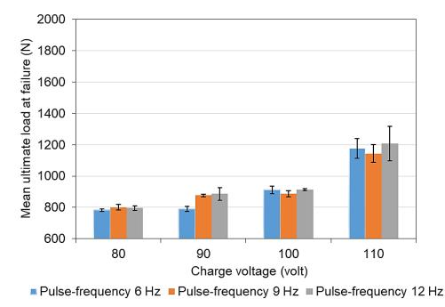
**Figure 14.** Effect of laser parameters on ultimate load at failure ± standard deviation (SD) (length of welding 5 mm).
