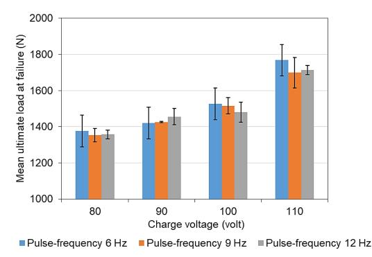
Figure 15. Effect of laser parameters on ultimate load at failure ±SD (length of welding 10 mm).
