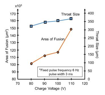
Figure 12. Effect of charge voltage on area of fusion and throat size.
