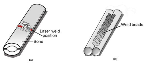
Figure 3. Type of proposed cerclage (a) cerclage wire (double loop) and (b) specimen with laser welding.
