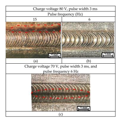
Figure 8. Weld appearance (a) Oxidation, (b) Good appearance with nice ripples, and (c) Lack of fusion.
